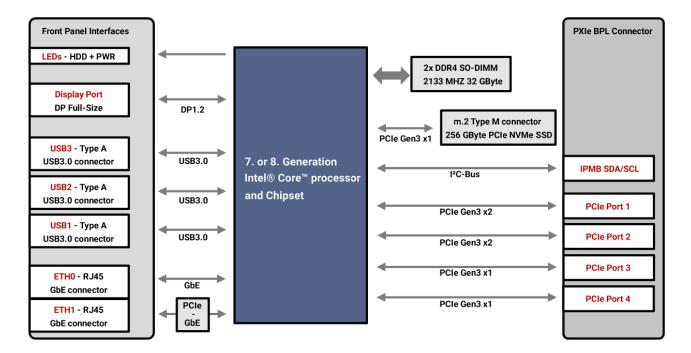
The nVent SCHROFF PXI Express embedded controller provides the following interfaces and connectors at the front panel:
